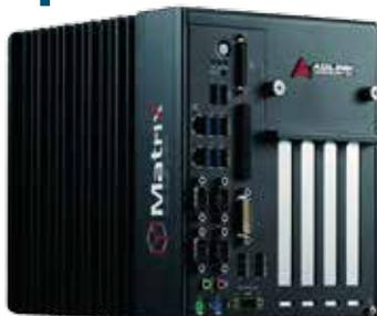
The Operator Work Stations (OWS's) are type-approved PC's with a solid state hard drive and Windows Embedded operating system, all to ensure a long mean time before failure. These OWS's can be controlled with a keyboard, trackball or touchscreen display.
